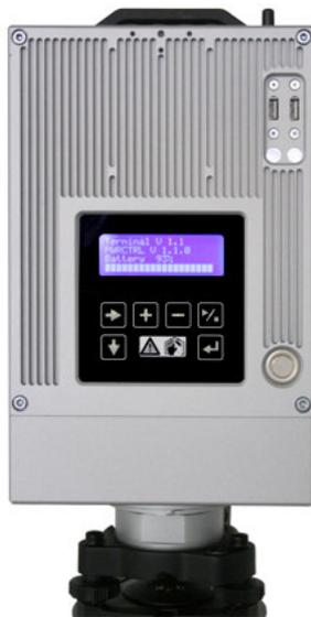
The imaging 3D laser measurement systems are applicable in the fields of digital planning of factories, industrial plants, architecture, protection of historic monuments, landscape and virtual reality. They are based upon the spot Z+F Laser Measurement System LARA:
